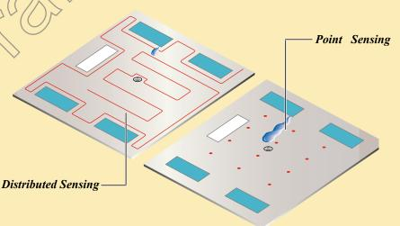
A TraceTek locating system detects the leak at its source, signals the alarm, and displays the exact position of the leak. By referring to a map of the system layout (supplied as part of the TraceTek system), you can quickly locate the leak source.
